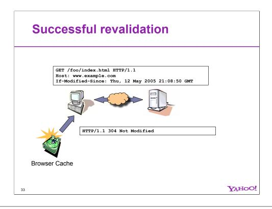
Apache simply stat()s the file and compares the timestamp to the If-Modified-Since timestamp. If the file's timestamp is less than or equal to the If-Modified-Since header, it returns 304 Not Modified.
